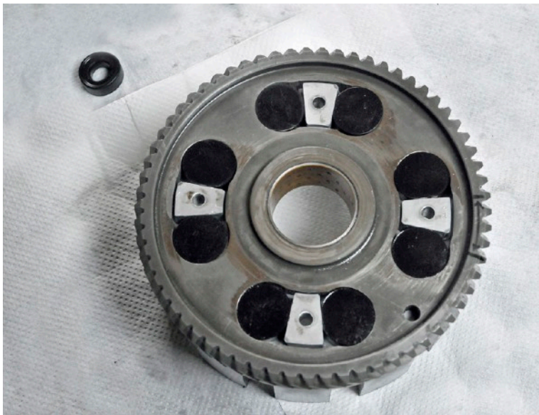
New discs in place
